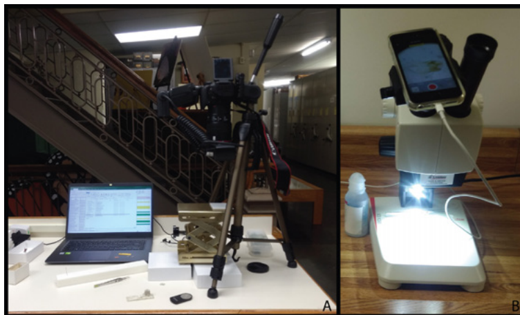
Figure 3. Photographic equipment: A. To photograph specimens; B. To photograph male genitalia.
