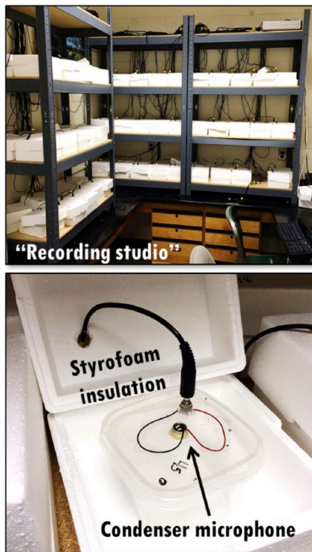
Figure 3. Custom-built sound relay equipment. Top photo is the entire array. Bottom photo shows one individual box. During call recording periods, one male resides in an individual box (which contains a lid-mounted condenser microphone) and is then placed within Styrofoam insulation to prevent cross-talk.
