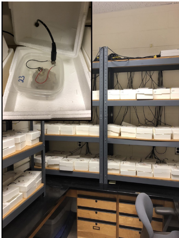
Figure 2. Individual calling boxes and room set-up. A) Males are placed in individual plastic containers with egg carton, food, and water to have their calls recorded. All boxes have a lid mounted microphone that relays back to the computer for measurement. B) Overall set-up of calling studio room, where over 100 individuals can be recorded at once.
